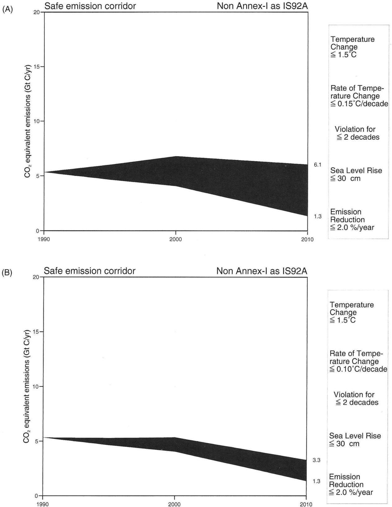
**Figure 2.** Two Annex-I emissions corridors for the EU objective with different rates of decadal temperature change: (a)  $0.15^{\circ}\text{C}$  per decade; (b)  $0.10^{\circ}\text{C}$  per decade.
